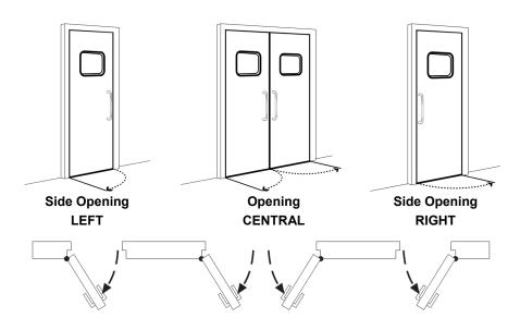
Side opening swing door (one leaf) or middle (two leaves). These can be manual or automatic with the incorporation of a surface motor group. If they are manual, each leaf can make sweep of up to 180°.
